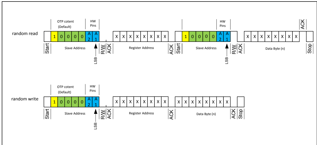
Figure 32: Slave Address Construction
